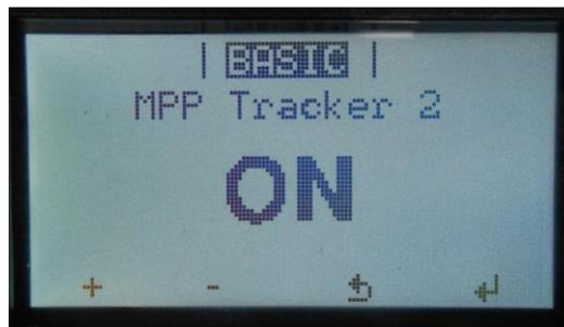
*Note: When the Fronius inverter is powered without the DC and the "MPP Tracker 2" is "ON", "INFO STATE 523 LOW PV VOLTAGE" will be displayed on the screen.*
