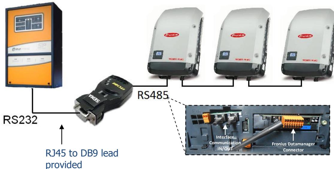
To install the Sena LTC100 adaptor, use the RJ45 to DB9 lead and connect the Sena LTC100 adaptor to the SP PRO Series I **Serial Port 2**. Then using 'CAT5' network cable or similar make, connect the Sena LTC100 adaptor to Fronius inverter 01 (Master) as per Table 1, Fronius Datamanager connector.
