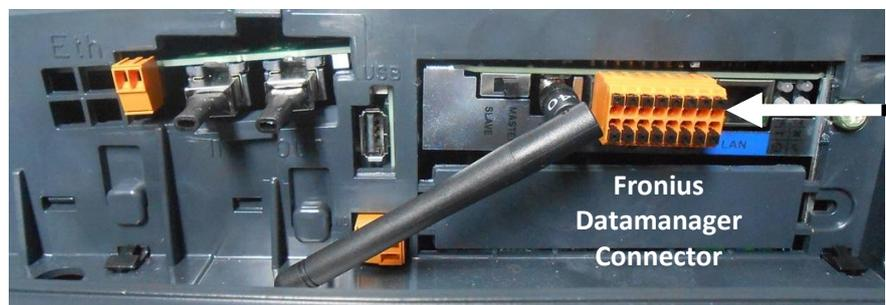
SP PRO Port 2 RJ45 connector to Sena LTC100 and to Fronius Datamanagement connector
